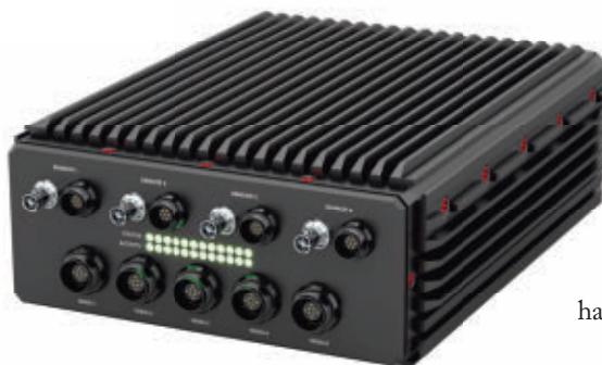
The General Micro Systems X9 module has the NVIDIA Jetson AGX Xavier or Orin CPU/GPU, and five 10 Gigabit Ethernet ports for inter-box communications, and multiple sensor inputs.
