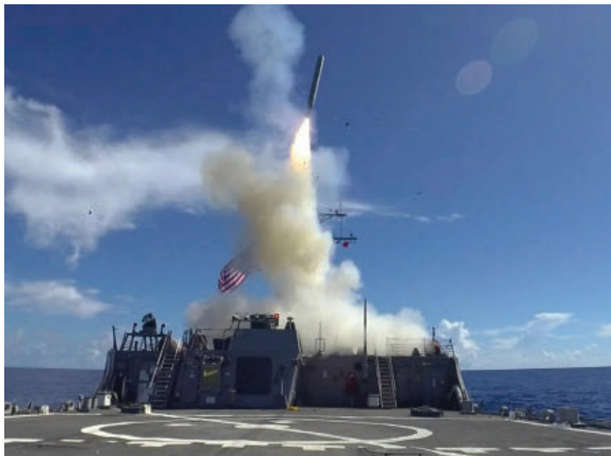
The tomahawk Block V uses an electro-optical sensor and radar altimeter to match nearby terrain to an internal database.
