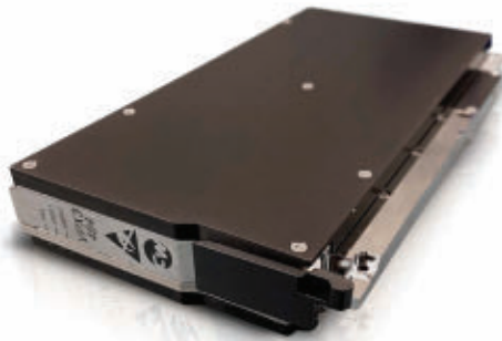
The Curtiss-Wright CHAMP-XD3/ is a 3U OpenVPX Intel Ice Lake Xeon D-1700 DSP processor card that features high-speed DDR4 memory, 10 Gigabit Ethernet, 40 Gigabit Ethernet Data Plane, and Xilinx Zynq UltraScale+ MPSoC FPGA for enhanced security.
